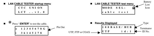
Use MODE/SEL to toggle between cable pin out screen and result display, press ESC back to test menu.
