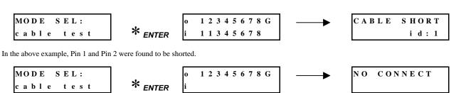
In the second example, if at least one pair of wires is not connected, the test result will show as "NO CONNECT".
