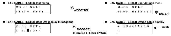
Use the **ENTER** key to set digits 1 to 8, G or blank (not connected), then press **MODE/SEL** to move to the next space. When completed, press **ESC**.(step no. 5 to 6)
