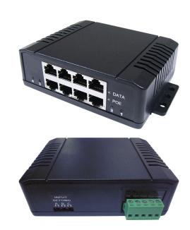
Equipped with bottom ports 1-4 on the front panel, RP-PGJ44GD follows a standard configuration, with data pairs and voltage distribution detailed for optimal performance. The unit supports data rates of 10M/100M/1000Mbps and operates within an input voltage range of 44 to 57V DC. With a maximum PoE power of 35W per port, RP-PGJ44GD incorporates robust protection features, including over-current and over/under voltage safeguards.
