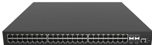
RP-PG83480I-4F is a Layer 2+ managed PoE switch. It offers 48 gigabit PoE ports and 4 1G/2.5G slots and delivers PoE power budget up to 740W. The switch provides full Gigabit access and exceptional scalability, offering impressive 2G performance. With a switching capacity of 144Gbps, it delivers high-density performance and includes Layer 3 static routing capabilities.
