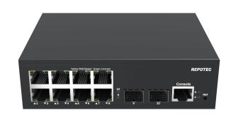
2\*1G/2.5G SFP ports. Its powerful Layer 2 management and high-performance switching offer a cost-effective Gigabit Ethernet solution for enterprise networks.
