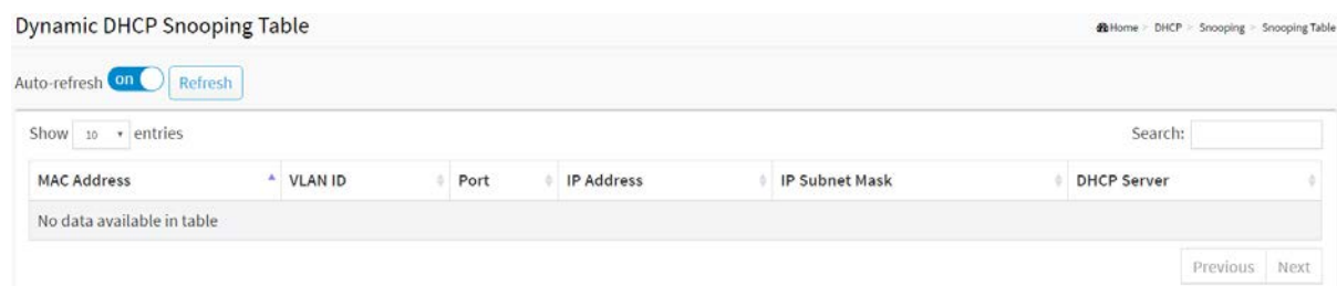
Figure 11-1.2: The DHCP snooping table
