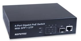
power, with a total PoE power budget of 65W (optional 120W). This switch is ideal for office users with a combination of PoE and non-PoE enabled devices, such as PoE IP Phones, Wi-Fi APs, and IP Cameras. It is IEEE 802.3af/at compliant, providing both power and data over a single cable.
