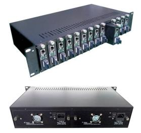
RP-MCR314 offers hot-swappable capability, allowing individual converters to be replaced or added without interrupting network connectivity. This flexibility enables easy upgrades or maintenance without affecting overall network operations. RP-MCR314 features a redundant power supply system, ensuring continuous and reliable power distribution. In the event of a power supply failure or maintenance, the redundant power supply seamlessly takes over, eliminating downtime and service interruptions.
