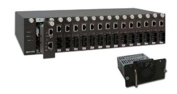
converters connected directly to the chassis's power backplane with a redundant power supply, When it contains two power supply units, if one fails, the other power supply starts running to keep the device powered up.
