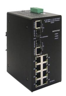
RP-ISF082G is a reliable and cost-efficient industrial Ethernet switch designed for various industrial applications, including factory assembly lines, automation systems, transportation, and heavy industrial factories. It meets the requirements of industrial applications, ensuring stable and uninterrupted operation
