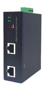
With a PSE input range of 15W to 90W, the RP-IPS0524 provides selectable output voltages of 5VDC, 6VDC, 12VDC, or 24VDC, configurable via a DIP switch, supporting current outputs of 2.5A or 5A. It is fully compliant with 60W uPoE and 95W Power over HDBaseT (PoH) standards, ensuring broad compatibility with various PoE configurations. RP-IPS0524 excels in adaptability, functioning as a reliable PoE solution even in the absence of a DC power source.
