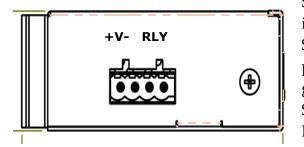
STEP 1 – Take out 4 pin terminal block located in the included mounting kit package.
