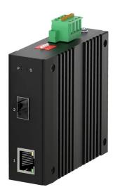
100/1000Base-X SFP, compliant with I IEEE802.3af/at PoE protocols, providing a maximum power consumption of 30W (PoE+). With convenient DIP switch configuration on the top panel, the device offers additional functionalities, including LFP, 100/1000M fiber port selection, 250m long-distance transmission support and PoE watchdog function.
