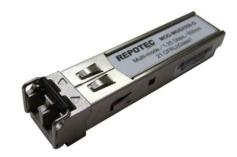
The transceiver consists of three sections: a FP laser transmitter, a PIN photodiode integrated with a trans-impedance preamplifier (TIA) and MCU control unit. All modules meet the standard of Class 1 Laser Safety.
