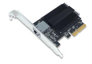
Cat5e/Cat6 or better cables. Designed with a low-power, low-profile PCIe small form factor and a single-port solution, the RP-4010EX enables widespread adoption of NBASE-T connectivity, resulting in a remarkable performance boost of up to 500 percent compared to Gigabit Ethernet speeds.
