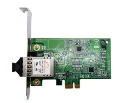
exceptional performance, it offers a maximum full-duplex bandwidth capacity of up to 2000Mbps, making it an ideal choice for high-end servers that require robust and reliable connectivity.
