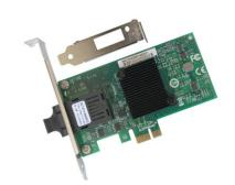
fiber LAN networks. This adapter complies with industry standards like IEEE 802.3z and 1000Base-X, offering a robust and reliable full-duplex bandwidth of up to 2000Mbps for high-end servers.
